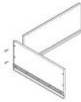
STEP 7: Fasten the Drawer Side Panel and Drawer Back Panel.
