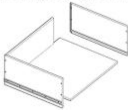
STEP 8: Insert Bottom and another Drawer Side Panel into the grooves.
