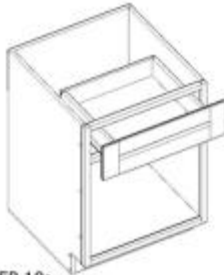
STEP 10: Slide the Drawer into the track.
