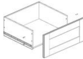
STEP 9: Position the Drawer Front into the grooves, then screw the Side Panel and the Front.
