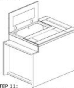
STEP 11: Fasten the hinges into the doors, then screw them on the cabinet.
