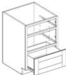
STEP 10: Slide the Drawer into the track.
