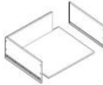
STEP 8: Insert bottom and another Drawer Side Panel into the grooves.
